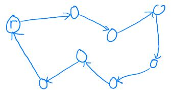
Very simple heuristic: find the cheapest connected subgraph T and do a depth-first traversal.
