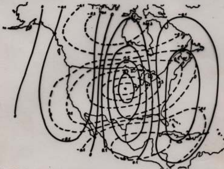
Figure 4.2.4.3: Isolines for the auto-correlation of the 500 mb u-wind component (dashed line) and the auto-correlation of the 500 mb v-wind component (full line). The "star" indicates the position of the reference station. (From Buel (1972)).
