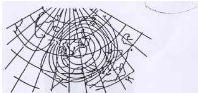
.: Isolines for the auto-correlations of the 500 mb geopotential between the station in Hannover and surrounding stations. From Bertoni and Lund (1963)
