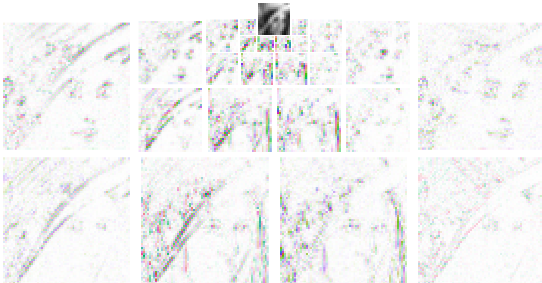
Figure 4: Four-level DT-CWT decomposition of Lenna into 6 subbands per level (only the central 128 \times 128 portion of the image is shown for clarity). A colour-wheel palette is used to display the complex wavelet coefficients.
